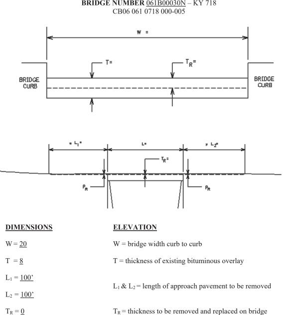
**BRIDGE DETAIL FOR PAVING PROJECT** BRIDGE NUMBER <u>061B00030N</u> – KY 718
