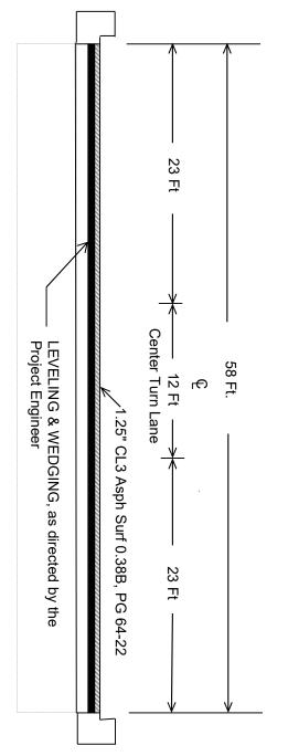
Asphalt Pavement Milling and Texturing Depth of Milling = 1.25 In.
