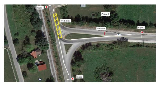
Phase 1 will have the northbound lane on US 31-W closed and traffic utilizing the southbound lane using a three phase signal. KY 224 westbound approach will be closed and traffic will utilize the eastbound approach during this phase.
