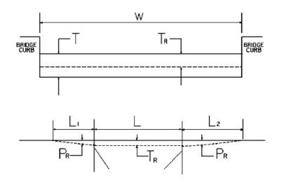
W = bridge width curb to curbT = thickness of existing bituminous overlayL = length of bridge $L_1 \& L_2$  = length of approach pavement to be removed $P_R$  = thickness to be removed and replaced on bridge $P_R$  = thickness to be removed and replaced on pavementNote:  $L_1 \& L_2$  lengths shall be determined by using a transition rate of 100 ft / inch of thickness $P_R$  = thickness
