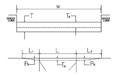
W = bridge width curb to curbT = thickness of existing bituminous overlayL = length of bridge $L_1 \& L_2$  = length of approach pavement to be removed $P_R$  = thickness to be removed and replaced on pavement $T_R$  = thickness to be removed and replaced on bridge $P_R$  = thickness to be removed and replaced on pavementNote:  $L_1 \& L_2$  lengths shall be determined by using a transition rate of 100 ft / inch of thickness
