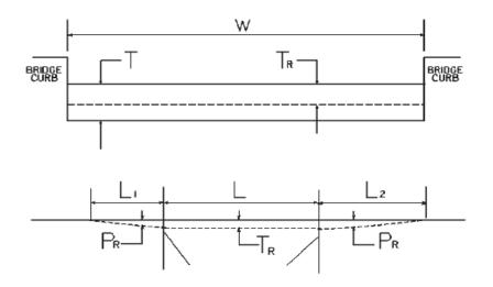
W = bridge width curb to curbT = thickness of existing bituminous overlayL = length of bridge $L_1 \& L_2$  = length of approach pavement to be removed $P_R$  = thickness to be removed and replaced on pavement $T_R$  = thickness to be removed and replaced on bridge $P_R$  = thickness to be removed and replaced on pavementNote:  $L_1 \& L_2$  lengths shall be determined by using a transition rate of 100 ft / inch of thickness
