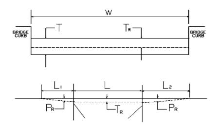
$\mathbf{W} =$  bridge width curb to curb  $\mathbf{T}$  = thickness of existing bituminous overlay  $\mathbf{L} =$ length of bridge  $L_1 \mbox{\&} \ L_2$  = length of approach pavement to be removed  $\mathbf{P}_{\mathbf{R}}$  = thickness to be removed and replaced on pavement  $\mathbf{T}_{\mathbf{R}}$  = thickness to be removed and replaced on bridge Note:  $L_1 \& L_2$  lengths shall be determined by using a transition rate of 100 ft / inch of thickness
