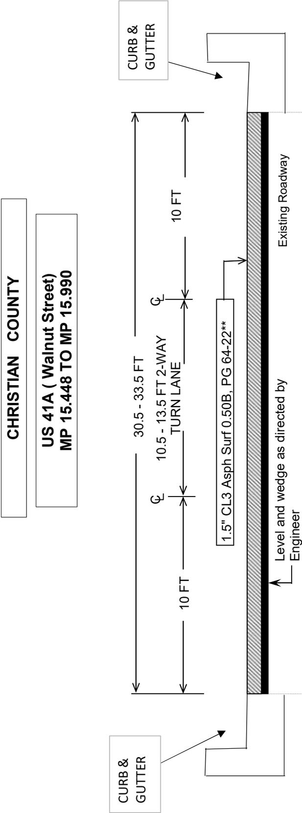
**\*3-LANE SECTION TAPERS DOWN TO 2-LANE BETWEEN THE 15.904 MM AND 15.95 MM**
