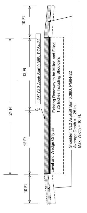
1.25 Inches Asph Milling and Texturing Max Width = 44 Ft
