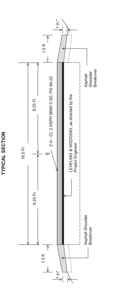
\*Where Existing Site Conditions Permit, DGA Base to be used as directed by engineer to eliminate drop offs. \*Edge of pavement to be tapered using the Durable Pavement Edge Shoe attachment
