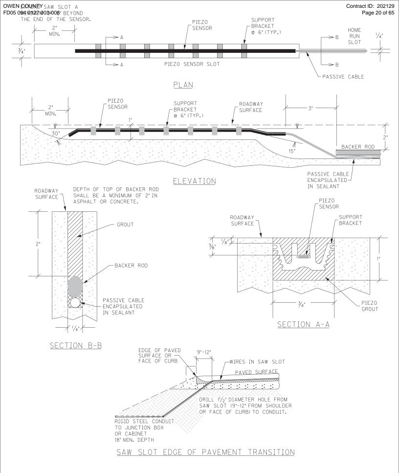
PIEZOELECTRIC SENSOR INSTALLATION
