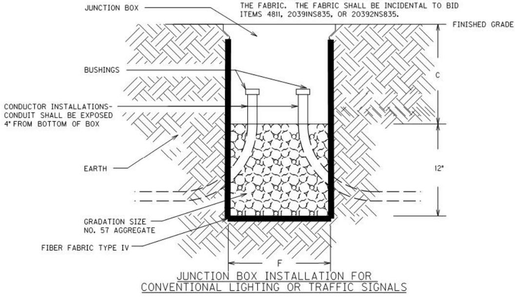
JUNCTION BOX INSTALLATION FOR CONVENTIONAL LIGHTING OR TRAFFIC SIGNALS
