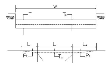
W = bridge width curb to curbT = thickness of existing bituminous overlayL = length of bridge $L_1 \& L_2$  = length of approach pavement to be removed $P_R$  = thickness to be removed and replaced on bridge $P_R$  = thickness to be removed and replaced on pavementNote:  $L_1 \& L_2$  lengths shall be determined by using a transition rate of 100 ft / inch of thickness $P_R$  = thickness
