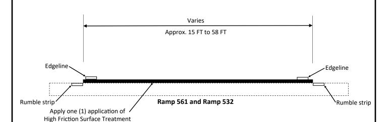
**Edgeline Rumble Strip Note:** The HFST should extend to, but not over, the shoulder rumble strip. Protect the shoulder rumble strip in accordance with the Special Note for Polymer Concrete Overlay-Systems.
