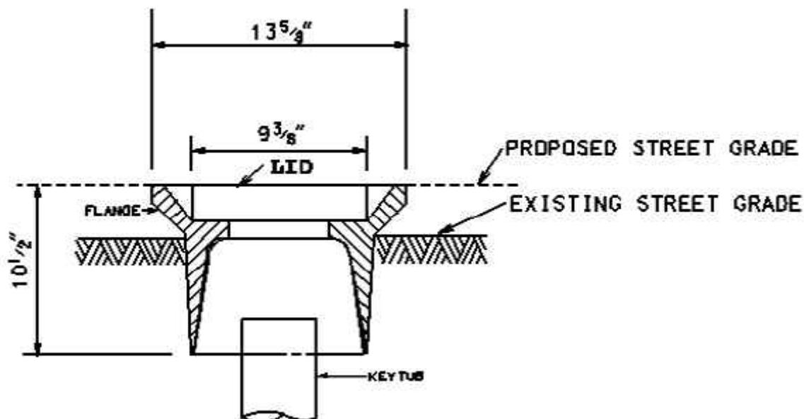
1. Unless directed otherwise by the Engineer, adjust all water valve boxes to grade during resurfacing operations. For streets to be milled prior to resurfacing, either mill around the valve box or remove the round top and replace it prior to paving as approved by the Engineer.
