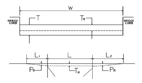
W = bridge width curb to curbT = thickness of existing bituminous overlayL = length of bridge $L_1 \& L_2$  = length of approach pavement to be removed $P_R$  = thickness to be removed and replaced on bridge $P_R$  = thickness to be removed and replaced on pavementNote:  $L_1 \& L_2$  lengths shall be determined by using a transition rate of 100 ft / inch of thickness $P_R$  = thickness
