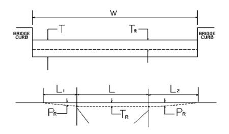
W = bridge width curb to curb  $\mathbf{T}$  = thickness of existing bituminous overlay  $\mathbf{L} =$ length of bridge  $L_1 \& L_2 =$  length of approach pavement to be removed  $T_R$  = thickness to be removed and replaced on bridge  $\mathbf{P}_{\mathbf{R}}$  = thickness to be removed and replaced on pavement Note: L1 & L2 lengths shall be determined by using a transition rate of 100 ft / inch of thickness
