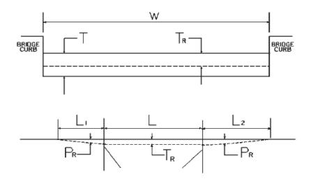
W = bridge width curb to curbT = thickness of existing bituminous overlayL = length of bridge $L_1 \& L_2$  = length of approach pavement to be removed $T_R$  = thickness to be removed and replaced on bridge $P_R$  = thickness to be removed and replaced on pavementNote:  $L_1 \& L_2$  lengths shall be determined by using a transition rate of 100 ft / inch of thickness
