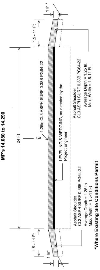
12.995 - 13.208: 12 foot driving lanes, 1.5' shoulders 13.208 - 13.23: Transition to 3 lane section, end paved shoulders. 14.00 - 14.29: 4 lanes, 12' width. 11' Paved shoulders TSPAVESURFACEshld surface shoulder.xls
