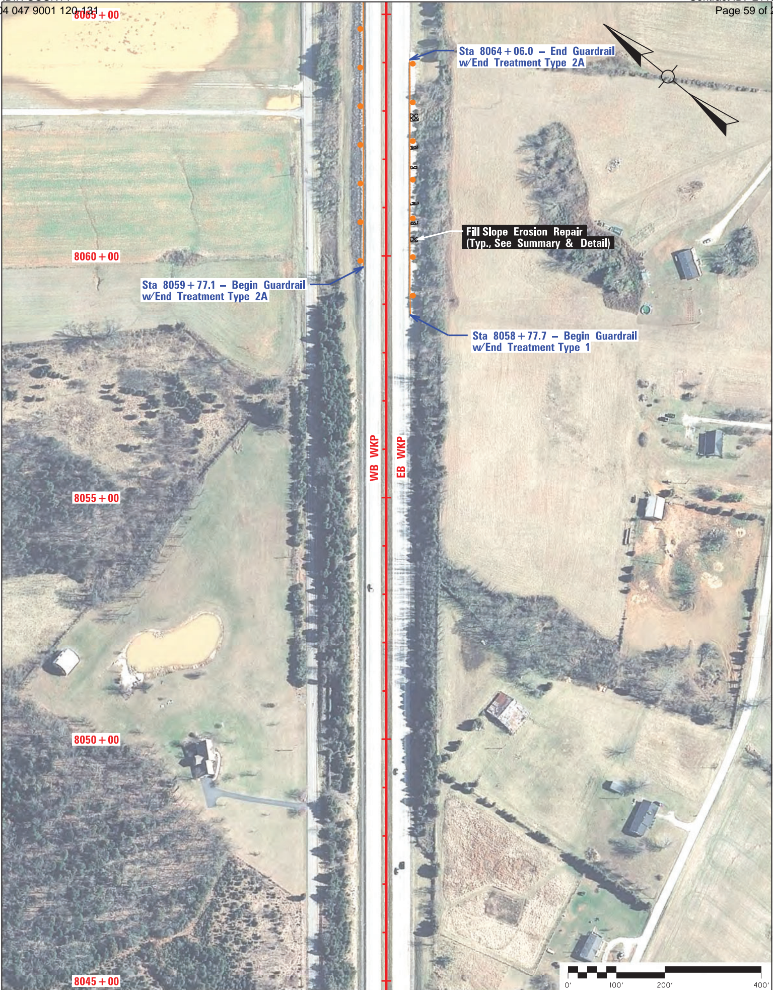
WKP (WK-900I) Rehab Plan - Scale 1" = 200' - Sheet 20 of 31 - Sta 8045+00 to Sta 8065+00
