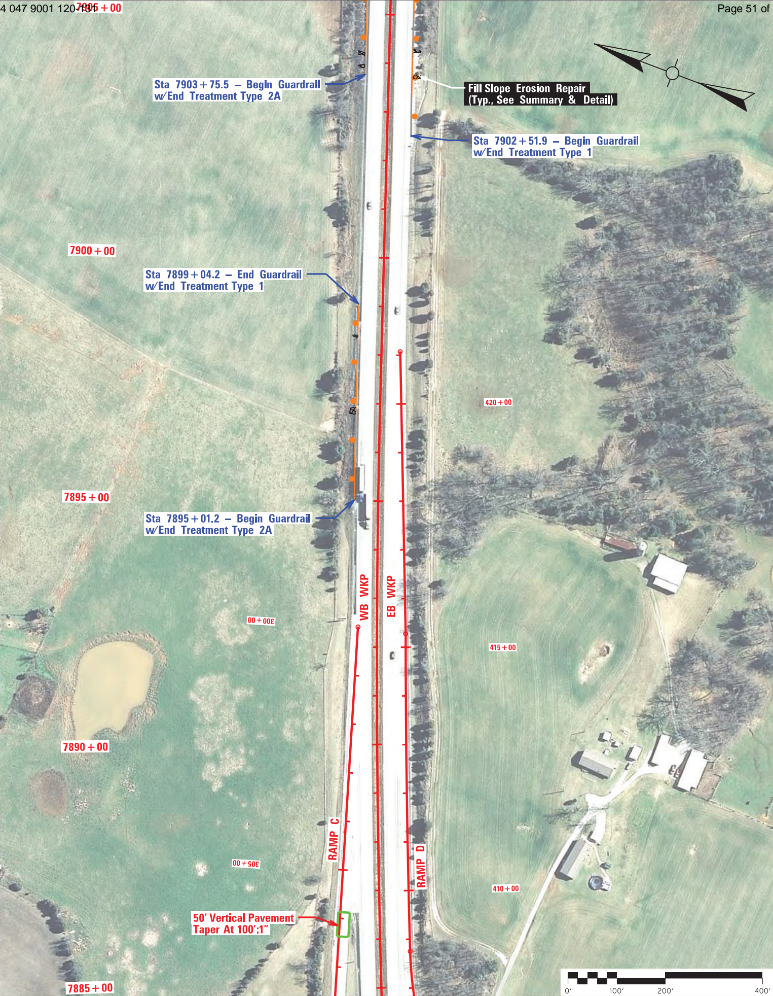
WKP (WK-900I) Rehab Plan - Scale 1" = 200' - Sheet 12 of 31 - Sta 7885+00 to Sta 7905+00
