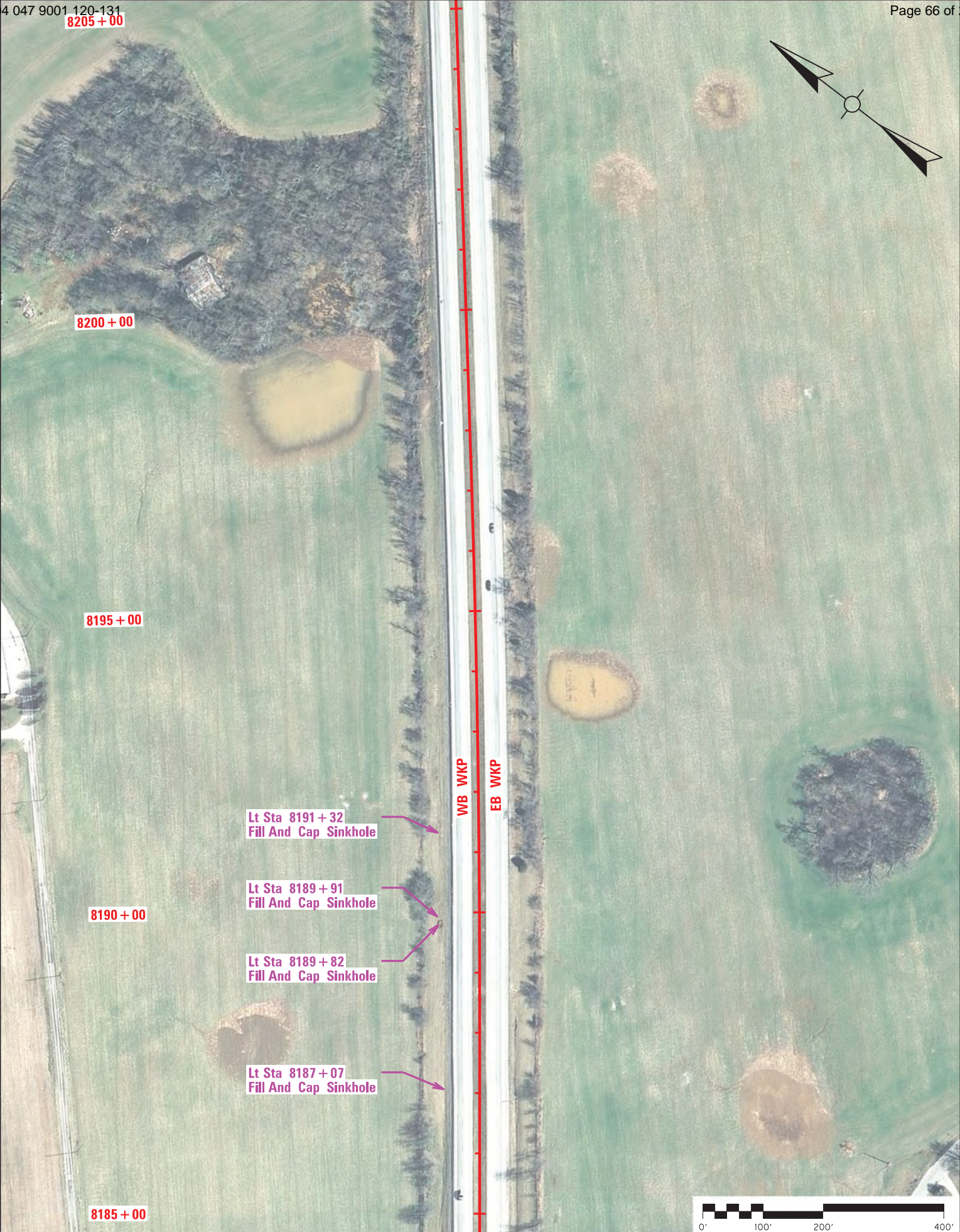
WKP (WK-900I) Rehab Plan - Scale 1" = 200' - Sheet 27 of 31 - Sta 8185+00 to Sta 8205+00
