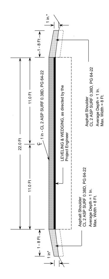
\*Where Existing Site Conditions Permit DGA to be placed where drop off is excessive, as directed by the Project Engineer
