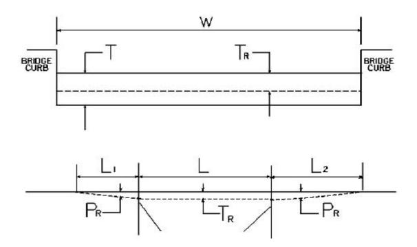
W = bridge width curb to curb T = thickness of existing asphalt overlay
