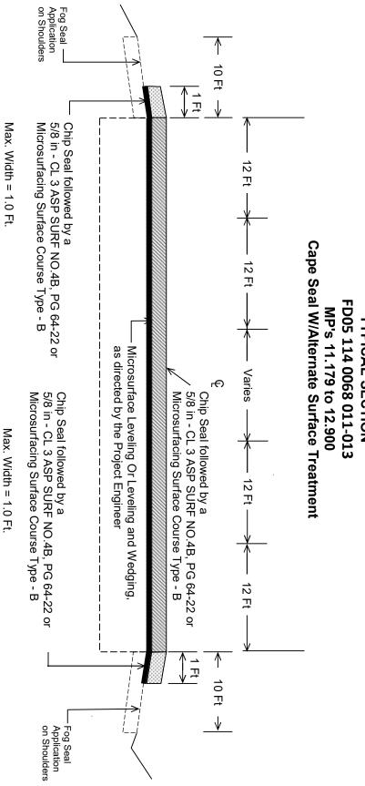
\*Where Existing Site Conditions Permit \*DO NOT DISTURB RUMBLE STRIPS \*TY V Pavement Marker Removal will be incidental to Asphalt Surface and will not be considered for payment.
