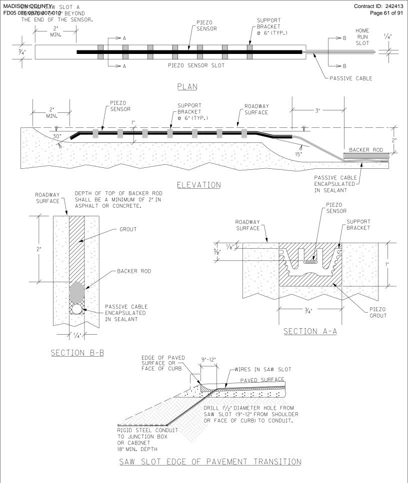
PIEZOELECTRIC SENSOR INSTALLATION
