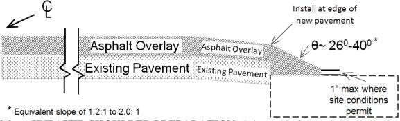
**2.0 UNPAVED SHOULDER PREPARATION.** Prior to placing asphalt pavement, prepare the shoulder material, including removal of vegetation/sod, where the pavement wedge will be placed to provide a foundation that will support the placement of the pavement wedge according to Section 403.03.02 of the Standard Specifications.
