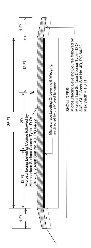
\*Shoulders to be pulled monolithically with mainline pavement.
