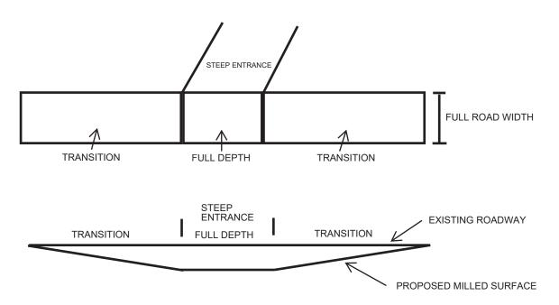
NOTE: THE TRANSITION LENGTH IS BASED ON 100 FT/INCH OF THICKNESS.
