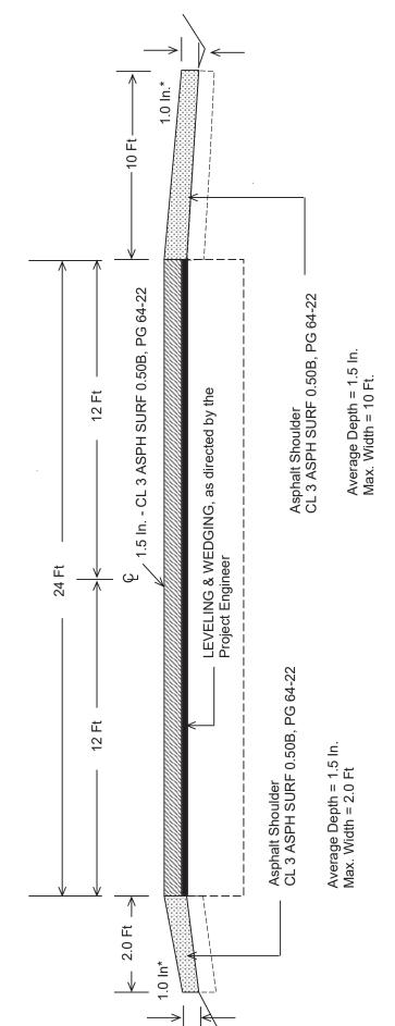
\*Contracor is to place 1.0ft wide DGA beyond edge of pavement with avg. depth of 1.5in. Where Existing Site Conditions Permit
