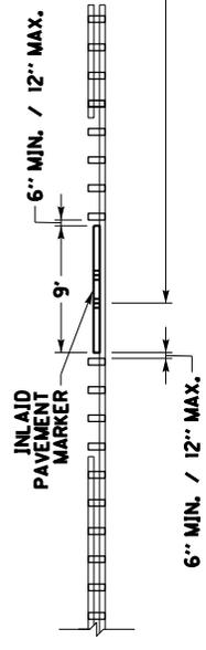
DETAIL FOR CENTERLINE RUMBLE STRIPS WITH INLAID PAVEMENT MARKERS
