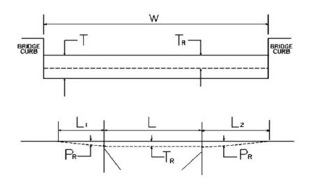
W = bridge width curb to curbT = thickness of existing bituminous overlayL = length of bridge $L_1 \& L_2$  = length of approach pavement to be removed $P_R$  = thickness to be removed and replaced on pavement $T_R$  = thickness to be removed and replaced on bridge $P_R$  = thickness to be removed and replaced on pavementNote:  $L_1 \& L_2$  lengths shall be determined by using a transition rate of 100 ft / inch of thickness
