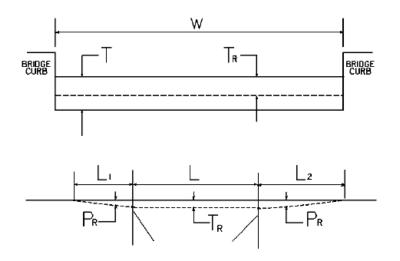
W = bridge width curb to curb  $\mathbf{T}$  = thickness of existing bituminous overlay  $\mathbf{L} =$ length of bridge  $L_1 \& L_2 =$  length of approach pavement to be removed  $T_R$  = thickness to be removed and replaced on bridge  $\mathbf{P}_{\mathbf{R}}$  = thickness to be removed and replaced on pavement Note: L1 & L2 lengths shall be determined by using a transition rate of 100 ft / inch of thickness
