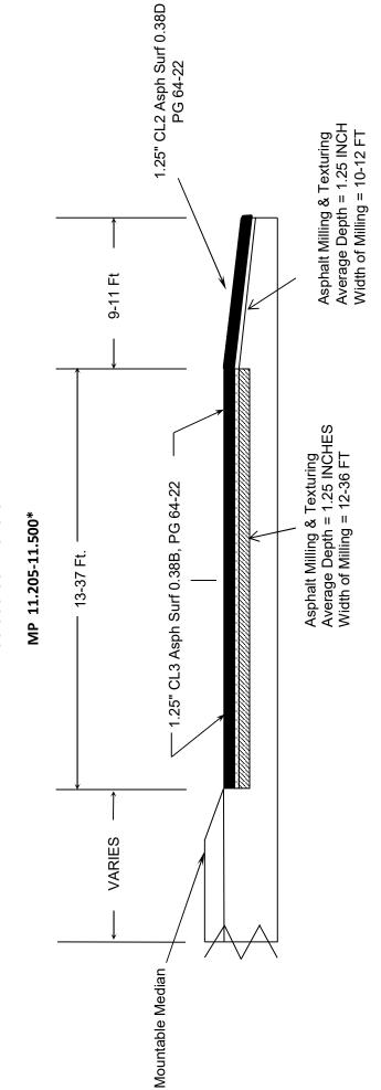
\*\*See Special Note for Proposed Mainline/Shoulder Surface Joint for more information about the new joint location. \*See Milling Summary Sheet for locations of all sections that shall be milled 1.25" full width.
