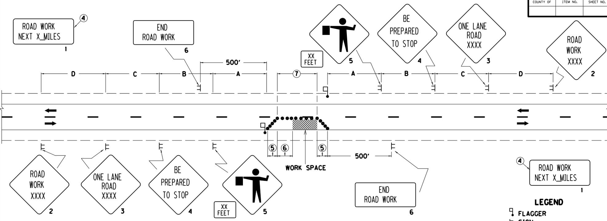
1. THE SIZE OF SIGNS 2 THRU 5 SHALL BE 48" X 48" WITH 30" X 24" SUPPLEMENTAL PLAQUES FOR EXPRESSWAYS/FREEWAYS. THE MINIMUM SIZE OF SIGNS 2 THRU 5 SHALL BE 36" X 36" WITH 24" X 18" SUPPLEMENTAL PLAQUES FOR OTHER ROADWAYS. SIGN NOS. 1 AND 6 SHALL BE 48" X 24" FOR EXPRESSWAYS/FREEWAYS AND 36" X 18" FOR OTHER ROADWAYS. A FREEWAY SHALL BE DEFINED AS A DIVIDED HIGHWAY WITH FULL CONTROL OF ACCESS. AN EXPRESSWAY SHALL BE DEFINED AS A DIVIDED HIGHWAY WITH PARTIAL CONTROL OF ACCESS.
