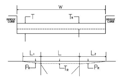
W = bridge width curb to curbT = thickness of existing bituminous overlayL = length of bridge $L_1 \& L_2$  = length of approach pavement to be removed $P_R$  = thickness to be removed and replaced on bridge $P_R$  = thickness to be removed and replaced on pavementNote:  $L_1 \& L_2$  lengths shall be determined by using a transition rate of 100 ft / inch of thickness
