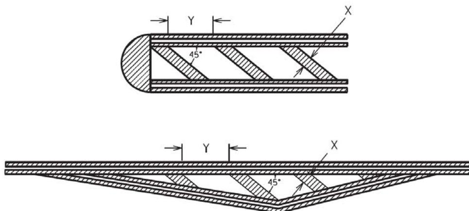
The cross-hatch pavement marking width (X) and spacing (Y) will usually be specified in the plans. The width to spacing values usually have a ratio of 1:10. If the plans do not specify the width (X) and spacing (Y) the Engineer will provide the contractor with the X and Y values for each cross-hatch installation. If necessary, the Engineer may obtain guidance from the District Traffic Engineer and/or the Division of Traffic Operations.
