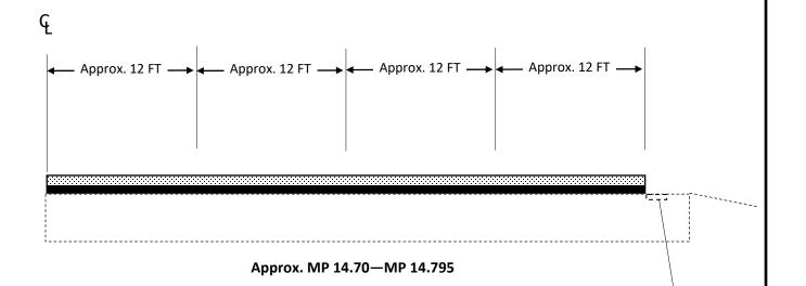
**Edgeline Rumble Strip Note:** The HFST should extend to, but not over, the edgeline rumble strip. Protect the edgeline rumble strip and edgeline pavement markings in accordance with the Special Note for Polymer Concrete Overlay Systems.
