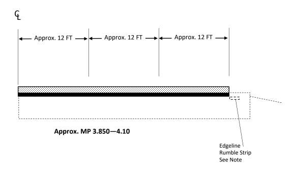
Edgeline Rumble Strip and Inlaid Pavement Marker Note: The HFST should extend to, but not over, the edgeline rumble strip and inlaid pavement markers. Protect the edgeline rumble strip, edgeline pavement markings, and inlaid pavement markers in accordance with the Special Note for Polymer Concrete Overlay Systems.
