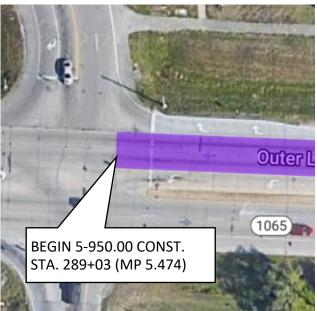
The beginning and ending points shown on this detail are approximate. The intent is for the High Friction Surface (HFST) to begin approximately 20 feet prior to the stop bar at Minor Lane, and end approximately prior to the exit from the businesses on the north side of the road. The Engineer shall mark the beginning and ending points for the HFST in the field at the time of construction.
