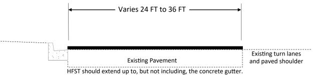
Cover and protect the edgeline and gore striping. Place HFST between the edgelines and/or gore striping.
