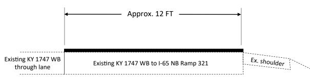
Cover and protect the edgeline and gore striping. Place HFST between the edgelines and/or gore striping.
