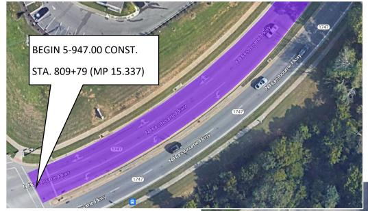
The beginning and ending points shown on this detail are approximate. The intent is for the High Friction Surface (HFST) to begin approximately 6 to 12 inches east of the crosswalk, and end near the median gore. The Engineer shall mark the beginning and ending points for the HFST in the field at the time of construction.
