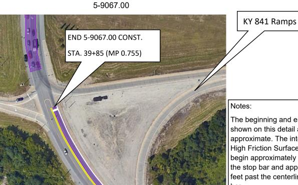
The beginning and ending points shown on this detail are approximate. The intent is for the High Friction Surface (HFST) to begin approximately 390' before the stop bar and approximately 10 feet past the centerline of the stop bar.
