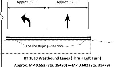
**Note:** Following HFST installation, install proposed lane line striping on top of HFST. If any sections of HFST are omitted due to pavement condition, continue proposed striping along the omitted section so that proposed striping covers the entire project limit.
