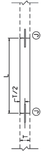
SECTION AA JOINT REPLACEMENT
