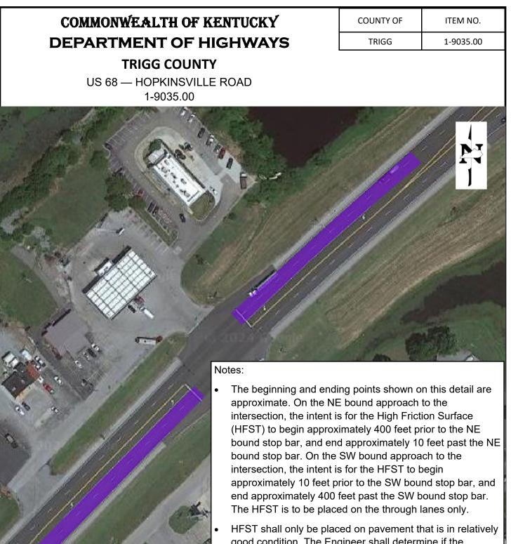
HFST shall only be placed on pavement that is in relatively good condition. The Engineer shall determine if the pavement is in acceptable condition prior to installing a HFST. If in doubt, the Engineer may contact CO HSIP staff to determine if pavement conditions have deteriorated significantly since the HFST site was identified.
