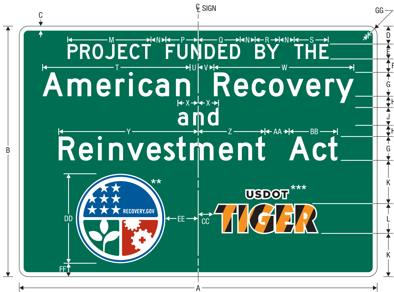
PROJECT FUNDING SOURCE SIGN
