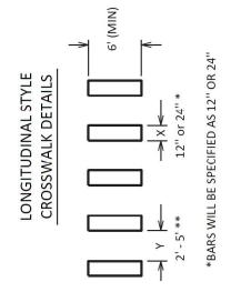
\*THE SPACE BETWEEN BARS IS TYPICALLY TWICE THE WIDTH OF THE BAR. ADJUST LAYOUT OF BARS AND/OR SPACING SO AS TO AVOID THE WHEEL PATHS OF APPROACHING VEHICLES. The longitudinal crosswalk bar width (X) will be specified in the bid item descriptions, summary sheets, and/or plans. The spacing (Y) between the longitudinal cross walk bars should be twice the bar width, unless otherwise specified, or otherwise directed by the Engineer:
