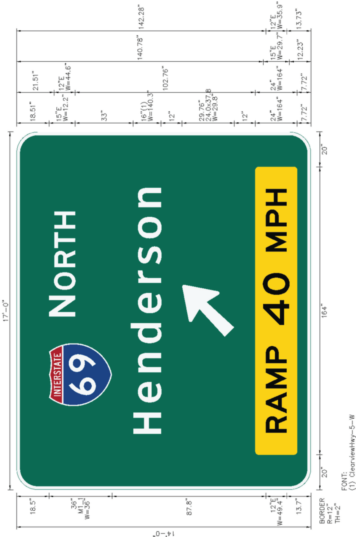
Graves County I-69 Ramp 241 MP 0.247 Sign Design Details for the Truss Mounted Sign over the RIGHT Ramp Lane
