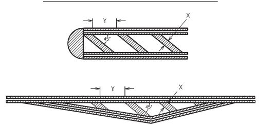
The cross-hatch pavement marking width (X) and spacing (Y) will usually be specified in the plans. The width to spacing values usually have a ratio of 1:10. If the plans do not specify the width (X) and spacing (Y) the Engineer will provide the contractor with the X and Y values for each cross-hatch installation. If necessary, the Engineer may obtain guidance from the District Traffic Engineer and/or the Division of Traffic Operations.
