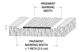
**3.2 Groove.** All grooves are to be positioned 2 inches from the respective pavement joint or as otherwise directed by the Engineer. In accordance with the above detail, the depth of the groove shall be 160 mils +/- 10 mils, and the groove width shall be one inch +/- ¼ inch wider than the width of the pavement marking to be placed in the groove.
