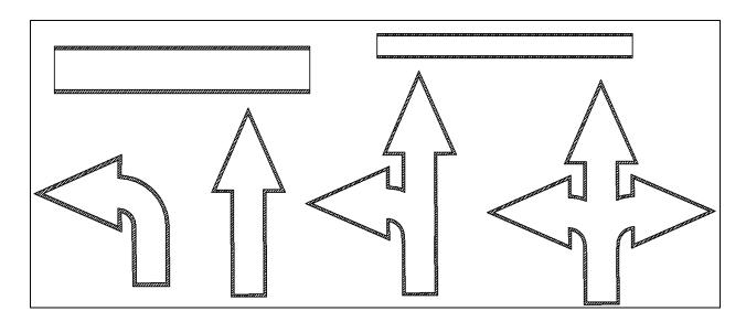
Contrast pavement markings shall consist of standard pavement markings with a defined contrast black border as shown in the chart below:
