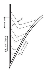
The chevron pavement marking width (X) and spacing (Y) will usually be specified in the plans. The width to spacing values usually have a ratio of 1:10. If the plans do not specify the width (X) and spacing (Y) the Engineer will provide the contractor with the X and Y values for each chevron installation. If necessary, the Engineer may obtain guidance from the District Traffic Engineer and/or the Division of Traffic Operations.
