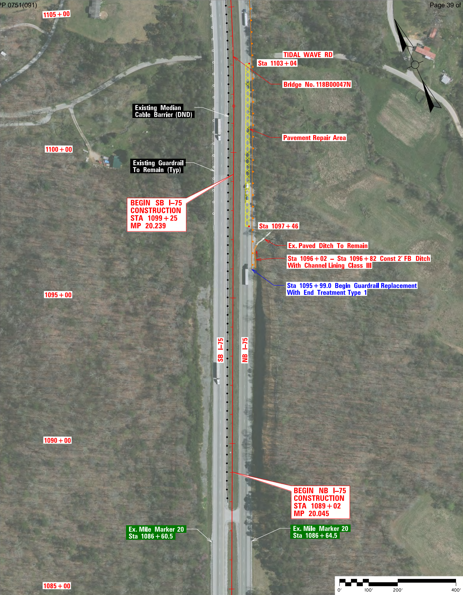
I-75 Rehab Plan - Scale 1" = 200' - Sheet 1 of 13 - Sta 1085+00 to Sta 1105+00
