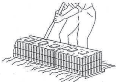
3. WEDGE LOOSE STRAW BETWEEN BALES
