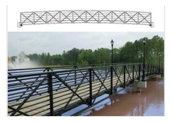
**3.5.1** Bridge(s) shall be designed utilizing either an underhung floor beam (top of floor beam welded to the bottom of the bottom chord) or an H-Section configuration
