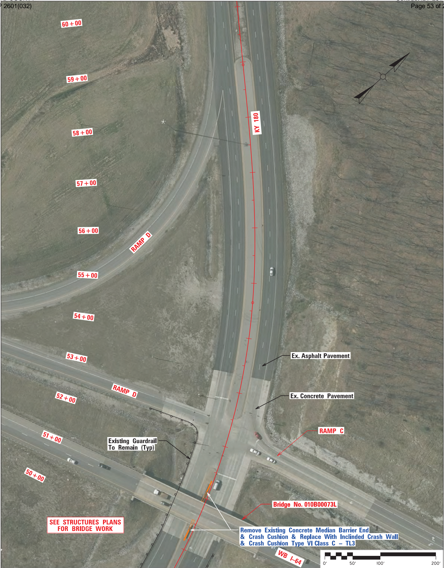
KY 180 Rehab Plan - Scale 1" = 100' - Sheet 6 of 14 - Sta 50+00 to Sta 60+00
