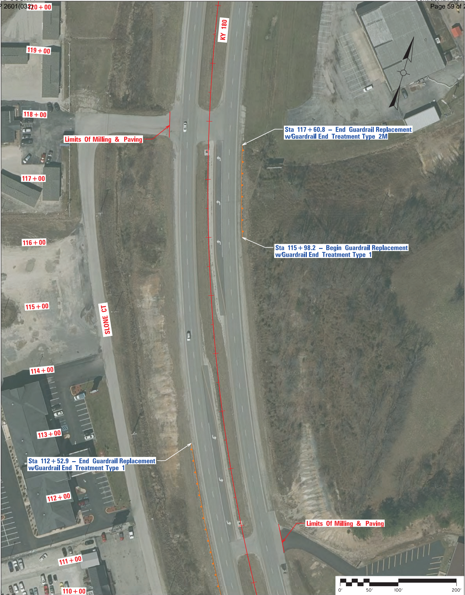
KY 180 Rehab Plan - Scale 1" = 100' - Sheet 12 of 14 - Sta 110+00 to Sta 120+00
