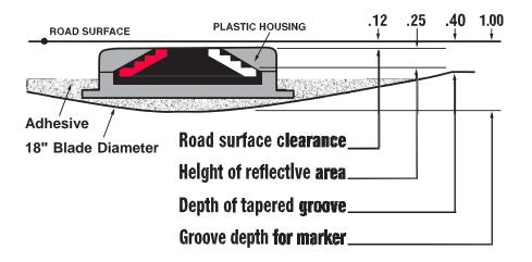
**D.** Location and Spacing. Install the markers in the pattern for high reflectivity with two (2) IPMs per groove. Locate and space markers as shown in the current standard drawings or sepias (note: use Inlaid Pavement Markers wherever Type V Pavement Markers are called for). Do not install markers on bridge decks. Do not install a marker on top of a pavement joint or crack. Offset the recessed groove a minimum of 2
