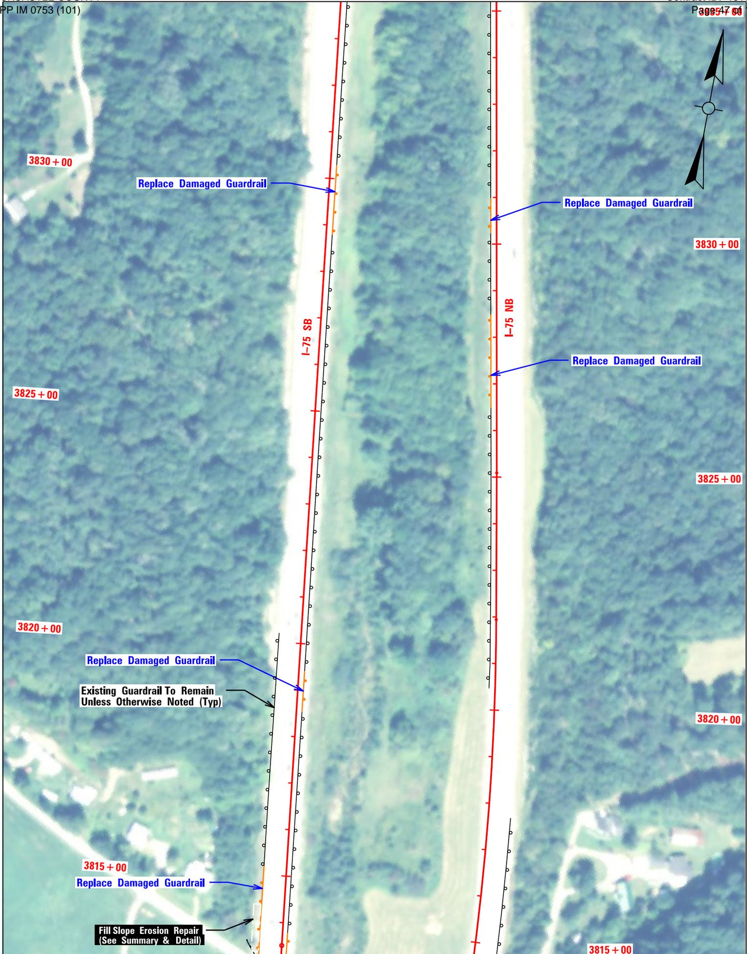
I-75 Rehab Plan - Scale 1" = 200' - Sheet 3 of 5 - Northbound Sta 3815+00 Sta 3835+00
